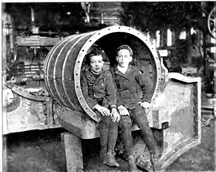
LOW PRESSURE CYLINDER, BALDWIN TWO-CYLINDER COMPOUND.
